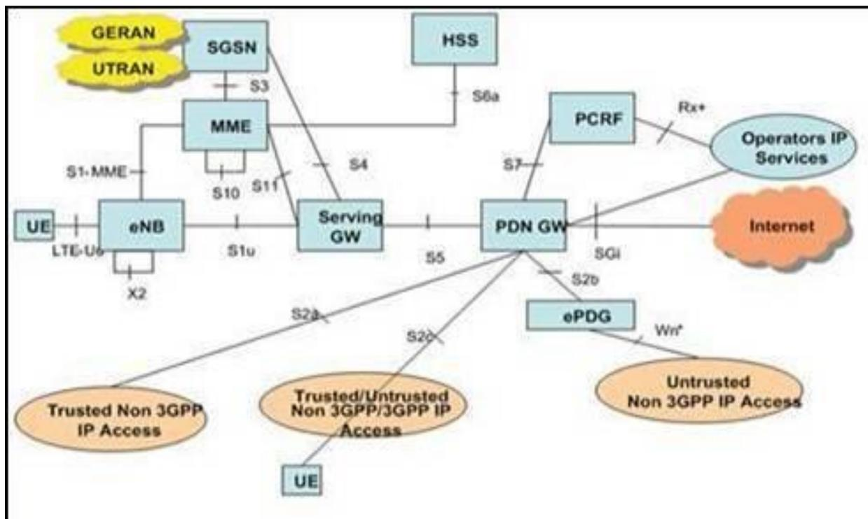
Figure-5: Non-Roaming Network Architecture for LTE for 3GPP accesses.
