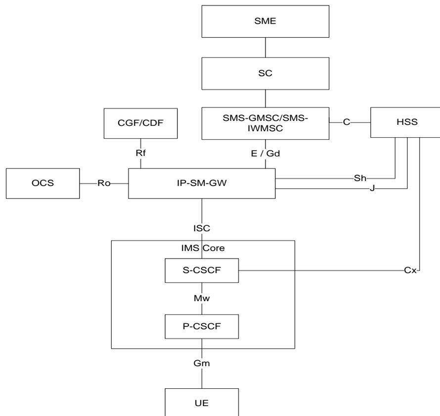
**Figure-12: SMS over Generic 3GPP IP access (3GPP TS 23.204).**
