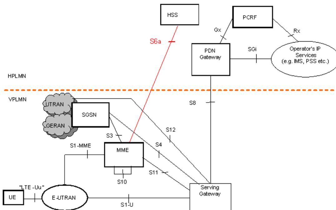
Figure-7: 3GPP LTE Roaming Architecture: Home-routed traffic using GTP based S8.
