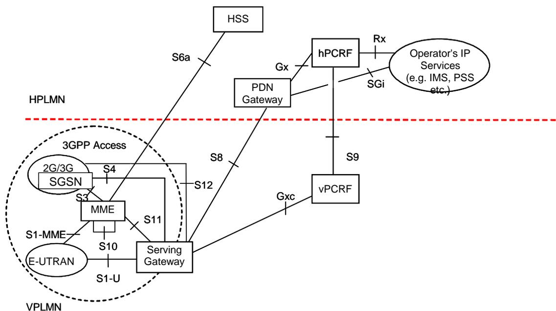
**Figure-8: 3GPP LTE Roaming Architecture: Home-routed traffic using PMIP based S8.**
