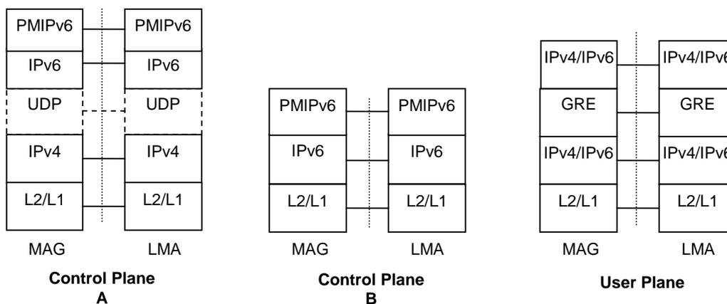
The Control Plane A is for PMIPv6 signals transported over IPv4, and the Control Plane B is for PMIPv6 signals transported over IPv6. When IPv4 transport is used, UDP encapsulation may be used as described in IETF RFC 5844.
