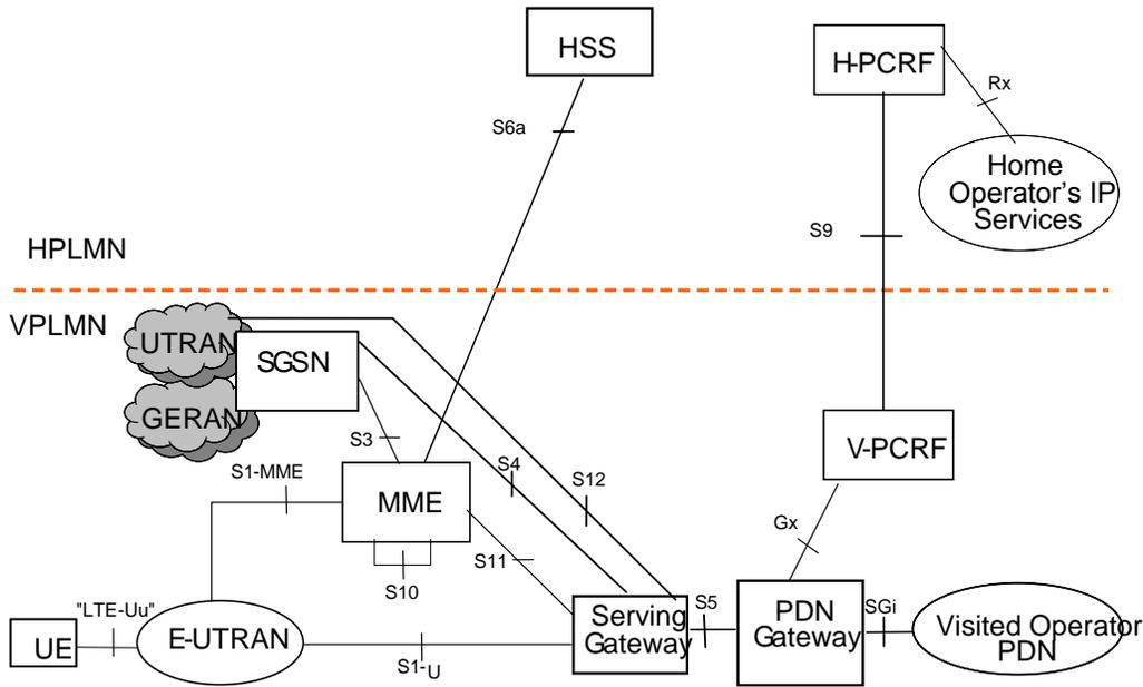
Figure-10: 3GPP LTE Roaming Architecture: Local Breakout using HPLMN operator functions.
