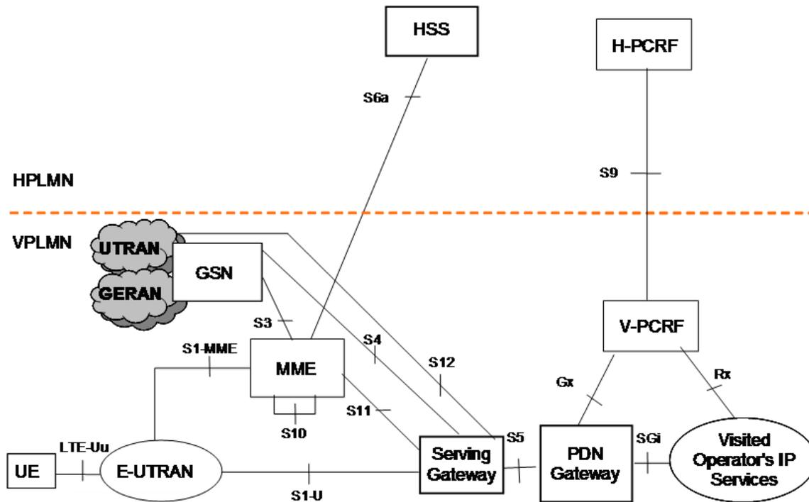
Figure-11: 3GPP LTE Roaming Architecture: Local Breakout using VPLMN operator functions.
