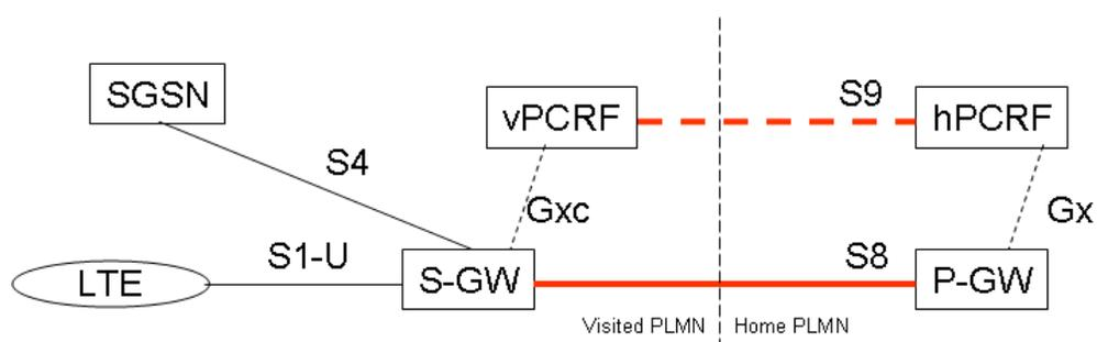
When PMIP-based EPC is used, the inter-operator interface will be S8 (PMIP) and S9 (PCC – Diameter). Policy and Charging Control (PCC) can be used if S8-PMIP is used. PCC allows EPC to provide more sophisticated QoS / Charging control. If PCC is not used, then PMIP provides no QoS and no S1 (or S4) bearer binding. Security requirements for PMIP are same as those of GTP.
